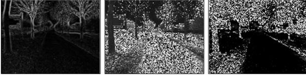
Figure 2. The image from Fig.1. after applying the Tamura features Coarseness (left), Contrast (middle) and Kurtosis (right).
